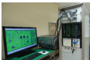
Precise inspection of electronic card using Pinpoint diagnostic equipment
