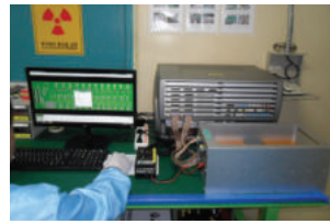
Precise inspection of electronic card
